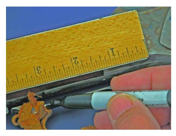
3. With the lever fully open, measure the distance between the two marks.
