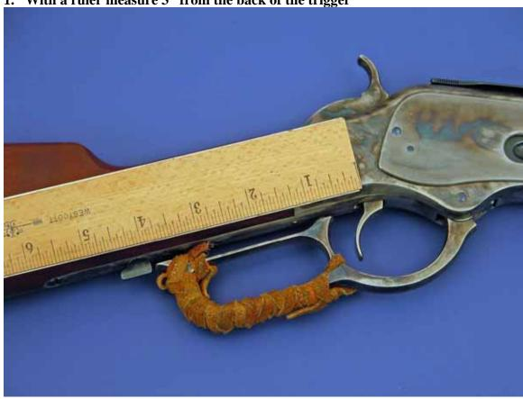
2. Mark the 3" position on both the receiver and the lever.
